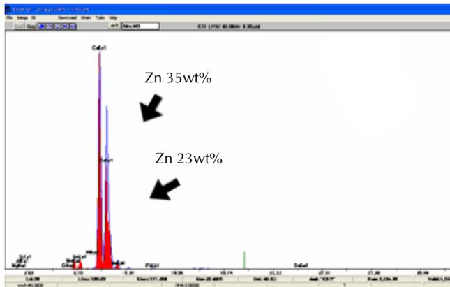
TRACER III-V: ARMI Cu Standards with Zn -- any work of art containing zinc outside of the historical boundaries of 28-32% zinc and no impurities would be suspect.<sup>3</sup>
