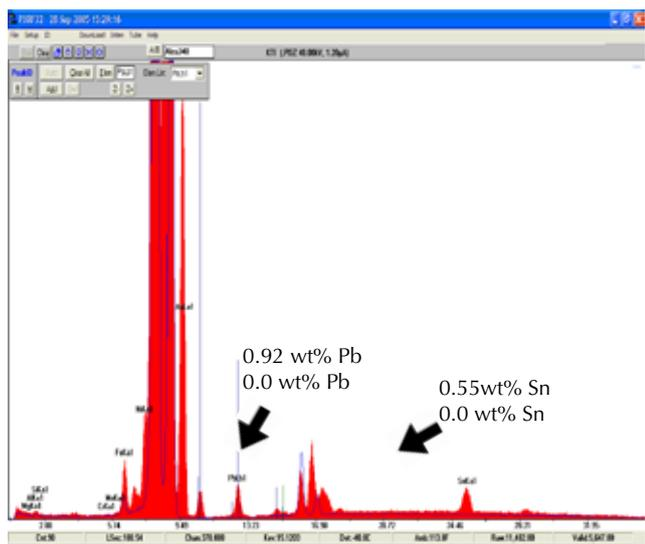
TRACER III-V: ARMI Cu Standards with Pb and Sn. The blue spectra contains no Pb or Sn compared with the red spectra containing 0.92% Pb and 0.55% Sn.
